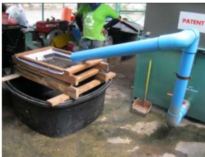
Figure 2.11: Filtering of digestate from Cowtec AD
