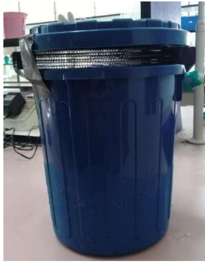
A prototype to attract female BSF to lay eggs.
